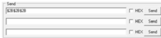
Send the transition frame in command mode in order to switch the device to configuration mode by clicking on the SEND button. After a few seconds, You must see the 2 LEDs light up permanently. On the com port terminal, you should also have "CM" feedback for Command Mode.
